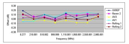
Additional analysis was done on the dynamic measurement uncertainty calculated for each measurement point. The uncertainties for each point at each station are shown in Figure 2. Note that the data clearly indicates an issue with one station at the low end of the frequency range. This was identified as a station issue and resolved.
