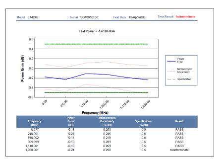
Figure 4. Offset or bias results in reduced margin at the highest frequency.
